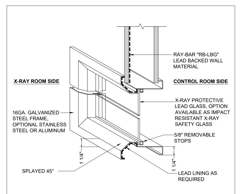
INNER FRAME TELESCOPES TO FIT WALL FROM 4 3/4" TO 7"
