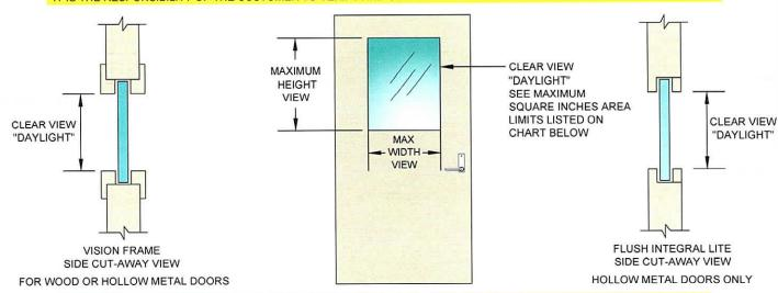
MAXIMUM CLEAR VIEW "DAYLIGHT" GLASS OPENING SIZES PERMITTED FOR FIRE RATED DOORS
