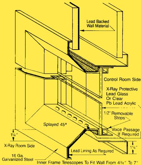
Rough Opening 1" Larger Than Glass Size On Control Side & 2 3/4" Larger On Splayed Side (2" Larger In Height For Frames With Voice Passage)
